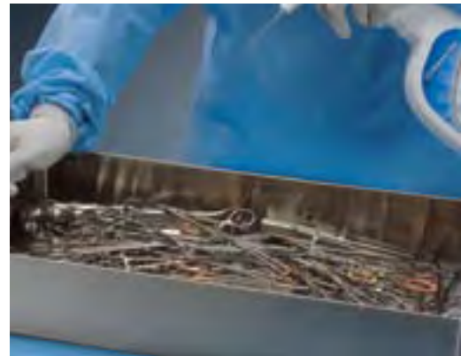
Proper device preparation aids in exposing all device surfaces to the cleaning solution.
